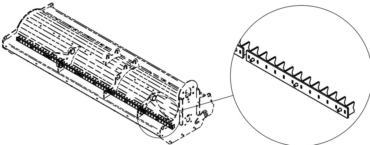
The mulcher can be mounted against steel (optional equipment). This is for finely chopping light materials such as grass.
